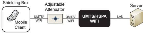
Fig. 4. Test Bed for Measurements of Power Consumption and Throughput
