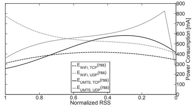
Fig. 5. Comparison of Power Consumption for UDP/TCP based Applications via UMTS/WiFi based on normalized RSS (1:=good, 0:=bad)
