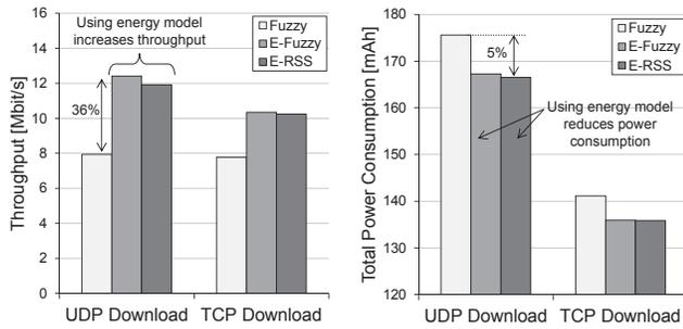
Fig. 8. Comparison of E-RSS and E-Fuzzy to the reference VHDA Fuzzy without Energy Model. Results are based on a Simulation where a Client needs 10 Minutes to reach the Target Point.
