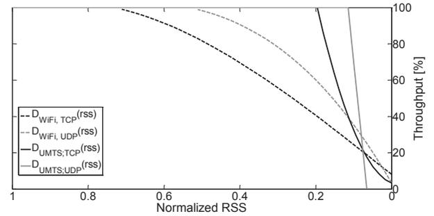
Fig. 6. Comparison of Throughput for UDP/TCP based Applications via UMTS/WiFi based on normalized RSS (1:=good, 0:=bad)
