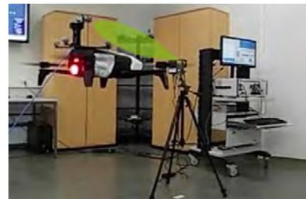
Figure 2: Indicated pencil beam from ground station and horn antenna on UAV in flight
