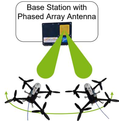
Figure 1: The ground station applies beamforming, whereas the UAV needs to only coarsely align by azimuthal rotation.
