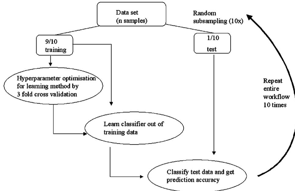
**Figure 6** Schematic workflow of predictor building, crossvalidation and optimization by support vector machines
