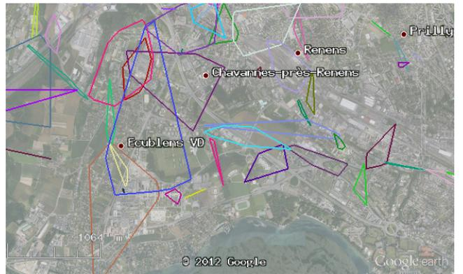
**Figure 2: Cell coverage plot based on GPS measurements of one user**
