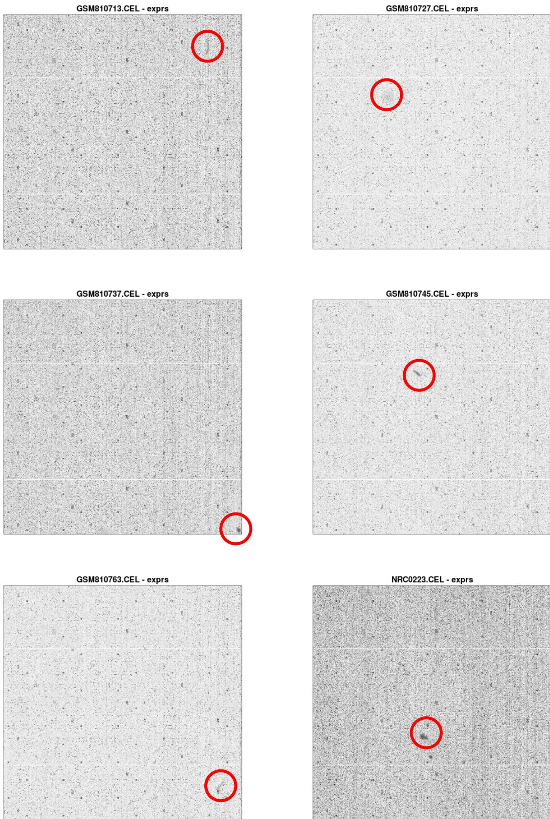
These chips with artifacts are discarded from any further processing, so that they would not affect RMA processing, for instance, in the following sections.
