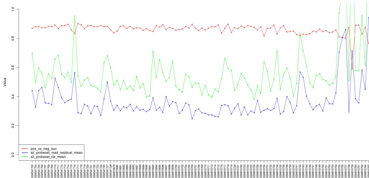
Overall, the auc values (red curves) are higher in Essen chips (mean 0.86) than in Amsterdam chips (mean 0.83), although Essen chips look much brighter than Amsterdam chips. Considering the typical auc values in 0.8~0.9, we choose the threshold rule ( $\text{auc} < 0.8$ ) to detect low-quality arrays. Here are the lists:
