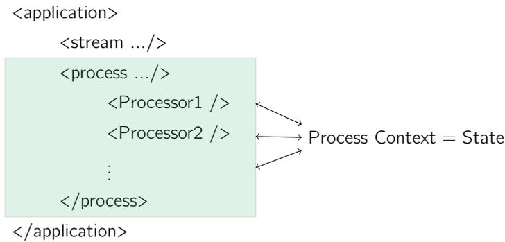
**Figure 39:** `streams` supports stateful processing by saving information inside a process context.
