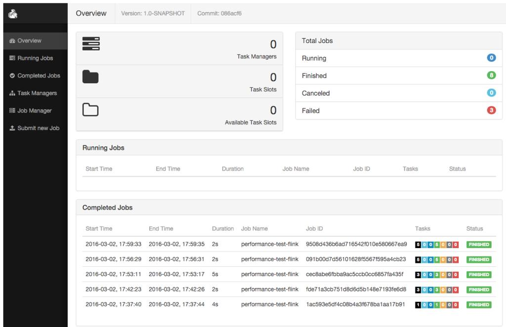
**Figure 22:** Web dashboard in Flink with pieces of information of the cluster and running and completed jobs.
