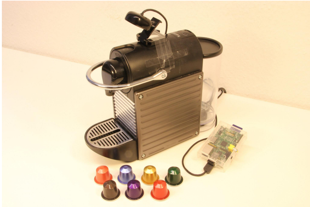
Figure 4.1.: The experiment set-up for the coffee capsule project. A web cam, installed on the coffee maker, continuously films the closing lever of the machine. If a capsule is inserted, the event can be detected and the capsule can be classified by its color. The web cam is connected to a computer, processing the incoming video data and making it available over TCP/IP.
