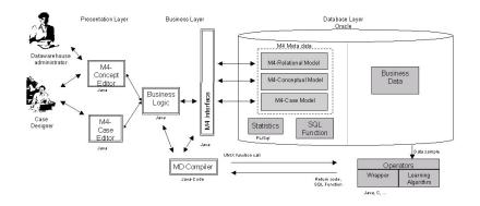
Schematic view of the Mining Mart architecture. The Concept Editor and Case Editor are part of the HCI. The M4 Interface provides a Java object interface to the M4 and is divided over the client (Java Swing) and the application server (JBoss). The Compiler (Java RMI server) executes operators and creates resulting tables and views. The database (Oracle) contains the M4 and the business data.
