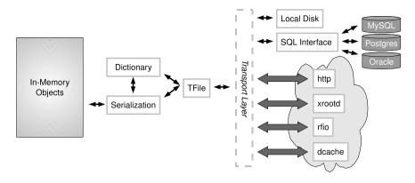
Fig. 3. Transient/persistent conversion in ROOT.
