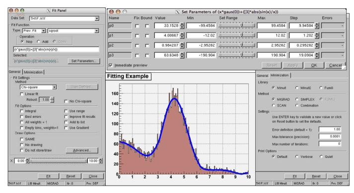
Fig. 7. The ROOT fit panel: the General tab (left) for selecting function, fit methods and options, the Set Parameter dialog (up right) for setting initial values and limits, and the Minimization tab (bottom right) for selecting the minimization library and method.
