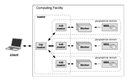
Fig. 10. PROOF multi-tier master-worker architecture.
