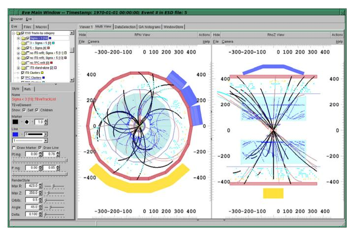
Fig. 9. Screenshot of AliEVE showing a simulated proton-proton event at the LHC collider as seen by the ALICE detector. The reconstructed particle trajectories are shown as black lines and the measured particle passage-points as colored dots.
